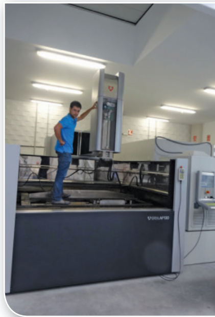
Fig #17 ONA AF130, the world's largest standard modular Wire EDM installed at Utimesa, an ONA customer located about an hour's ride from the Durango factory. This machine has travels of X 2,000mm, Y 1,300mm, Z 700mm. The machine will be used to cut components mainly for the energy industry. Note the garage door sized opening in the ceiling of the climate controlled EDM room to allow loading of parts via overhead crane.
