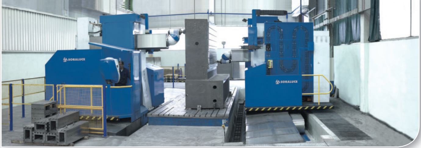
Fig #7 Machining an ONA Modular machine base. Note that the dual head machining center works on two opposite surfaces simultaneously.
