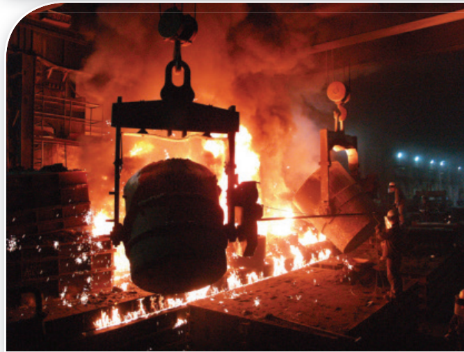
Fig #6 Pouring the casting for a large ONA machine tool base. For castings this large, a simultaneous pour from two crucibles is required.
