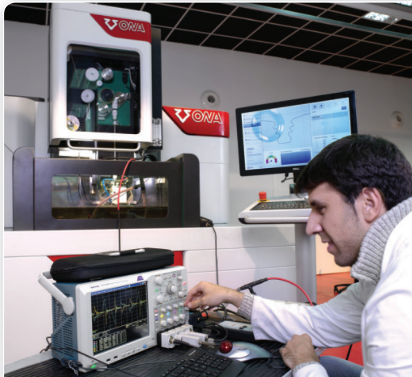
Fig #5 ONA engineer fine tuning the discharge pulses on the generator for their new AV25 Wire EDM
